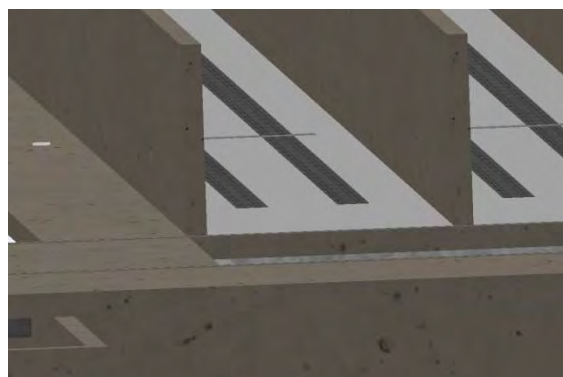
Photo 7 - Baseplate embedded in the bay floor
