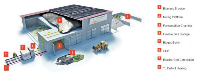
Example of Garage Style Dry Anaerobic Digestion Source: *BioFerm Energy Systems* http://biofermenergy.com/
