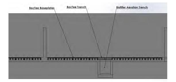
Photo 22 – Biofilter Detail
