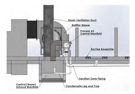
Photo 20 - Biofilter Drain Piping (typical)
