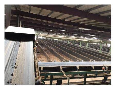
Photo 1 – Automated Overhead Bay Loading Telescoping Conveyor
