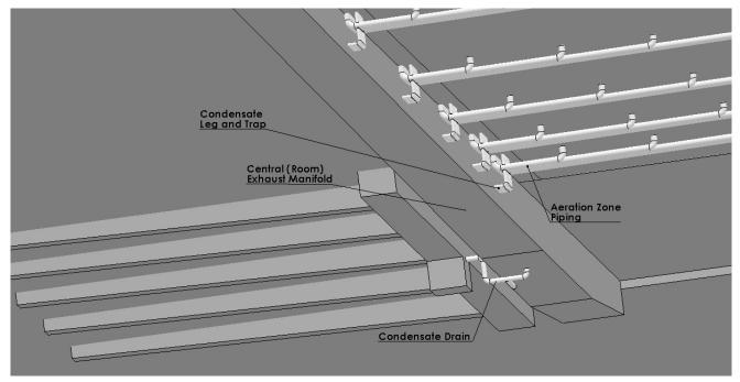
Photo 21 - Biofilter Drain Piping (typical)
