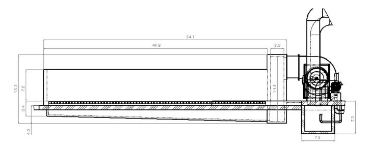
Photo 23 – Biofilter Cross Section
