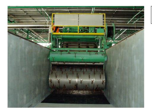
Photo 5 – Agitator over BacTee Aeration Floor The AgitatAeR<sup>™</sup> aeration control system (system) allows continuous modulation of process air based on temperature feedback from the process material. The aeration zones in each set of bays are linked by a common below-grade manifold to a blower for that particular zone. Thus for the five (50) total aeration zones, (10) aeration blowers are being supplied.
