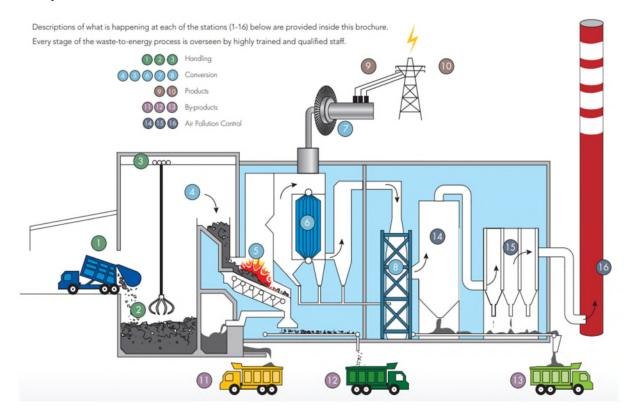
The process of generating electricity in a mass burn waste-to-energy plant has seven stages:
