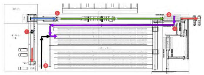
The biosolid receiving bay is convenient and easy to use. The pump truck opens its valves and drops the biosolid into a receiving hopper. Then, the **pumping/screw conveyors** drop the biosolid onto pre-cleaned organic matter and gets mixed into the BDP compost bays.
