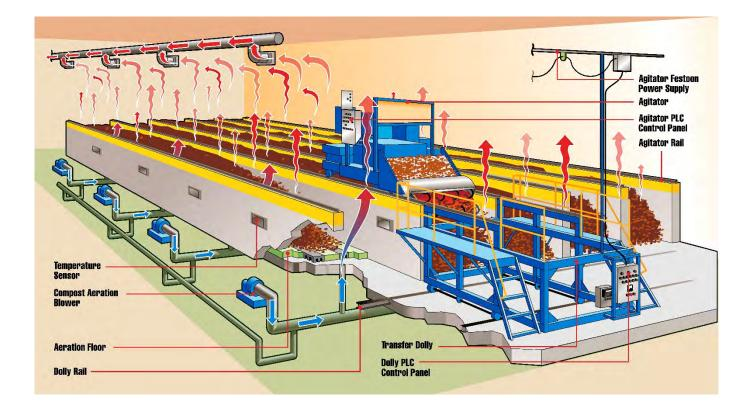
**Step 1 – Bay Loading –** The OSW and Biosolids will be blended prior to being delivered to the ICS bays. The bays are designed to receive nominally 40 yds<sup>3</sup> of feedstock (or "charge") following an agitation. The front 20 ft of each bay is a non-aerated concrete pad designated as the "Loading Area" of the bays. As discussed above, the primary method of loading the bays will be via a Machinex supplied overhead conveyor as shown in Photo 1.
