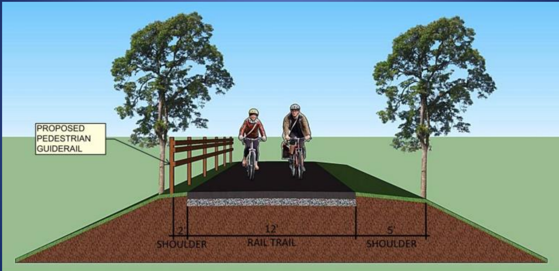
Figure 9 – Typical Section D (Guiderail and Standard Shoulder)
