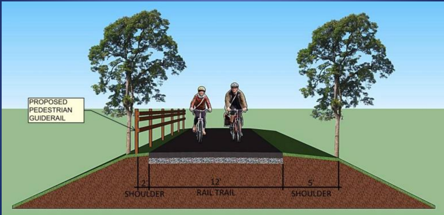
Figure 9 – Typical Section D (Guiderail and Standard Shoulder)
