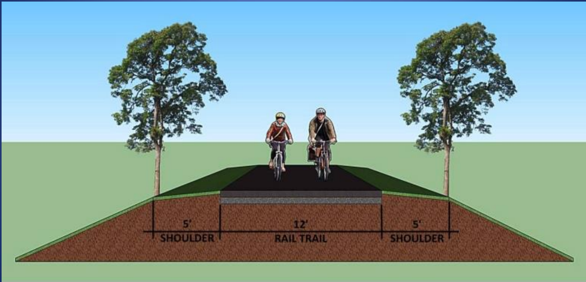
Figure 6 – Typical Section A (Standard Rail Trail Section)
