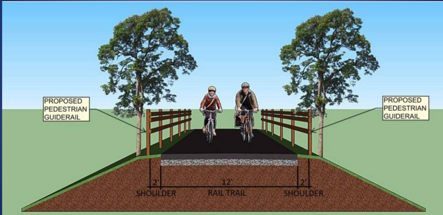
Figure 7 – Typical Section B (Rail Trail with Guiderail)
